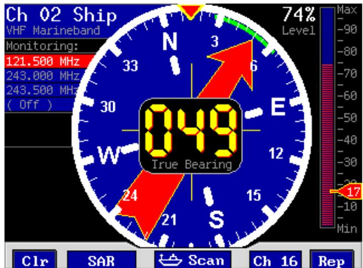
Fig. 4 Bearing operation
