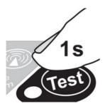
The rotary switch (8) is in position **ARM**. When pressing the button **TEST** (10) for about 1 second, The RT-B77 *HELB* will carry out a self-test procedure. It will check internal electronic parameters and the battery's condition.
