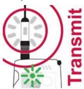
If the RT-B77 *HELB* is activated, the **white** function indicating LEDs (2) in the antenna and the **green** status LED (4) are blinking. After activation a sweeping sound can be heard for about 2 seconds. After 30 seconds the beacon ID will be indicated acoustically. During activation the sweeping tone of the distress signal modulation is given out every 30 seconds for duration of 2 seconds.
