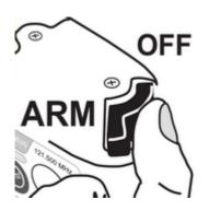
Turn the rotary switch (8) into position **OFF**. Now the RT-B77 *HELB* is switched off. The manual activator, the pull-away activator, the water contact and the test button are disabled. If there was a function active (standard, service, test) it will stop with the voice message: "**Power OFF**".
