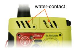
If the RT-B77 *HELB* is immersed into water for more than 10 seconds the PLB will be activated automatically. For that the water contacts behind the slots have to be bridged by water.
