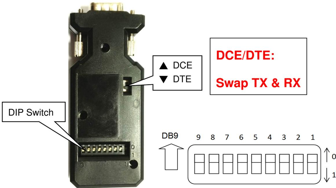
**2.4 Default: All pin is "0", Baud rate 9,600 bps., 8 Data bits, None parity, 1 Stop bit.**
