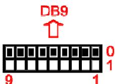
**2.5 Baud rate option: DIP No. 8 is set to “1” (On): The baud rate is 115,200 bps, 8 Data bits, None parity, 1 Stop bit.**
