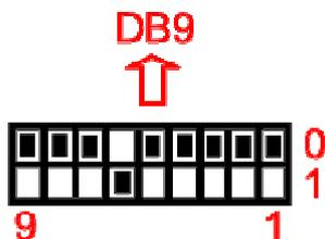
3.11 TPMS APP for ID setting: DIP No. 1 & 6 is set to "1" (On) and "0" else, Add "AT\$SNDTXT=" with TPMS packet as the section 3.10
