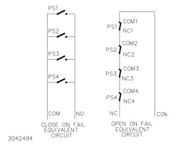
FIGURE 4. TYPICAL ALARM CIRCUIT DIAGRAMS
