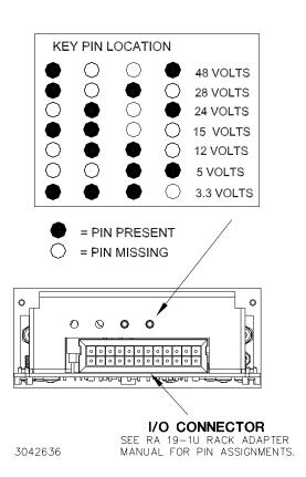
FIGURE 3. REAR CONNECTOR AND KEYING
