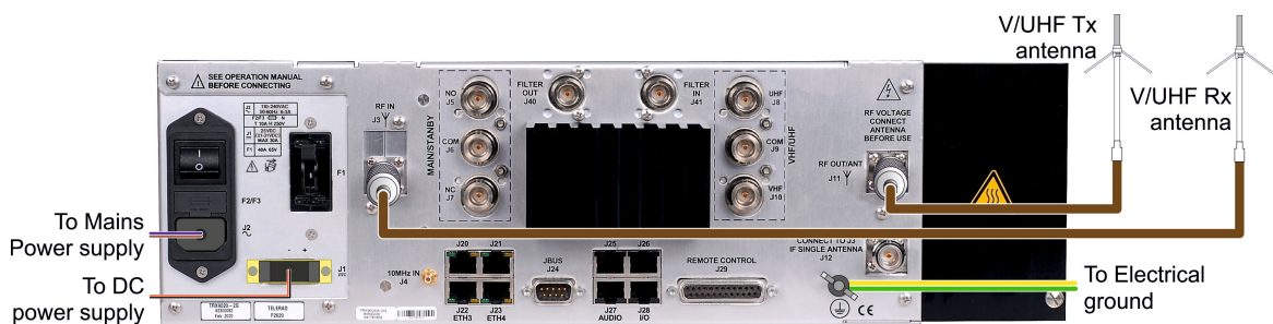
Figure 28 : Two separated V/UHF Tx and Rx antennas architecture
