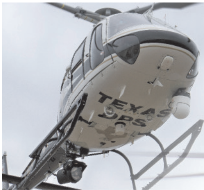
Law Enforcement version for bearing LoJack and ETS signals in addition to COSPAS-SARSAT and VHF emergency frequencies.
