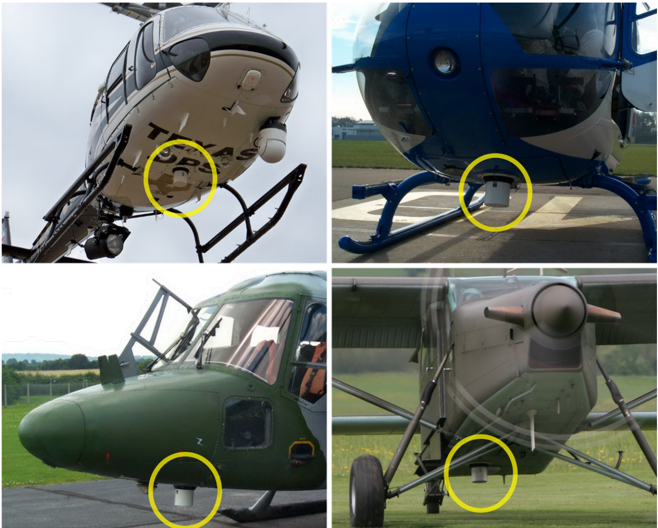
Fig 45) Antenna installed in good locations
