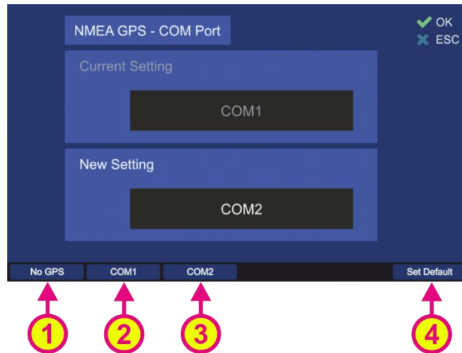
Fig. 157 NMEA GPS communication port settings
