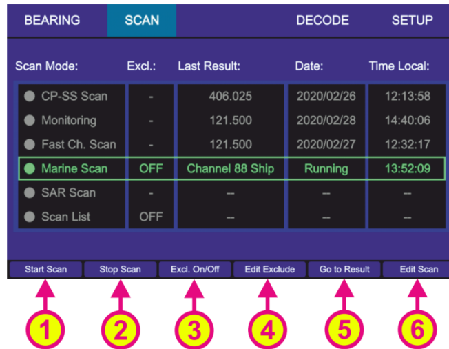
Fig. 41 Marine scan is activated
