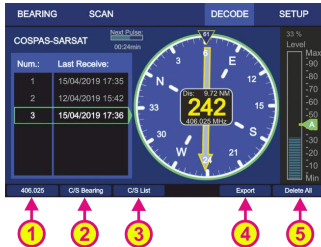
Fig. 63 "Decode" page. "Bearing and List" view
