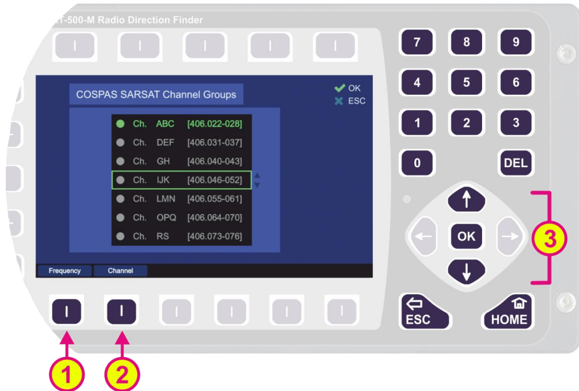
Fig. 14 Input of a new COSPAS-SARSAT frequency
