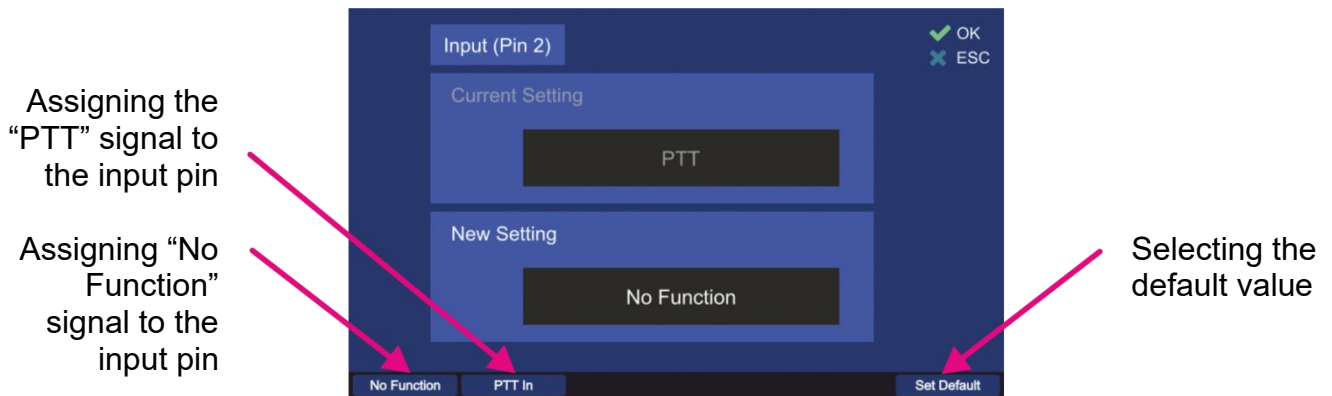
Fig. 160 Assigning a function to the input pin
