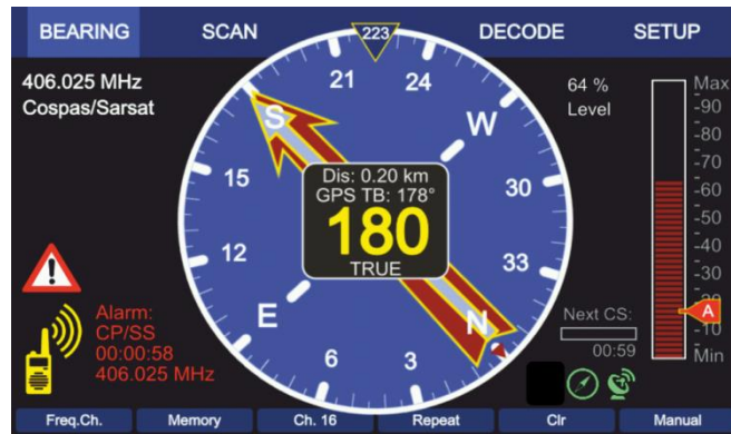
Fig. 64 Indication of the GPS based bearing on the Bearing page
