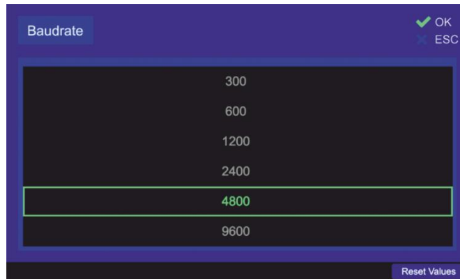
Fig. 158 Changing the NMEA GPS baud rate setting
