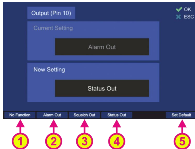
Fig. 161 Assigning a function to the output pin
