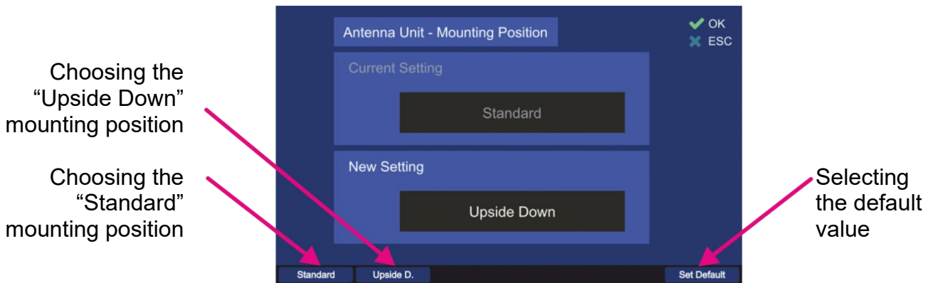
Fig. 112 Antenna unit (mounting position) dialog
