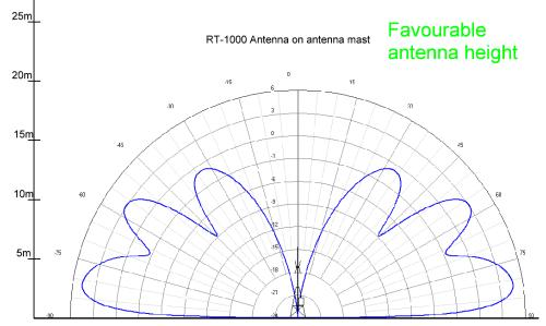
Ground reflections will cause the vertical antenna diagram having zeros, i.e. angles at which the sensitivity of the antenna is extremely low. Higher antenna positions cause more zeros in the vertical antenna pattern.
