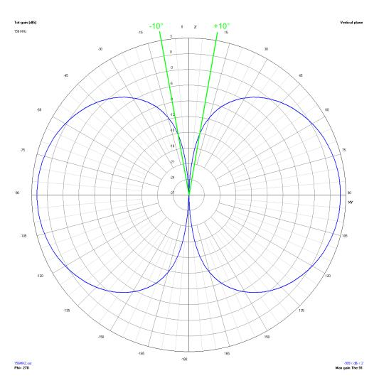
The graph above shows the free space vertical radiation diagram (antenna gain in dBi vs. vertical radiation angle) of a typical sea band dipole antenna.
