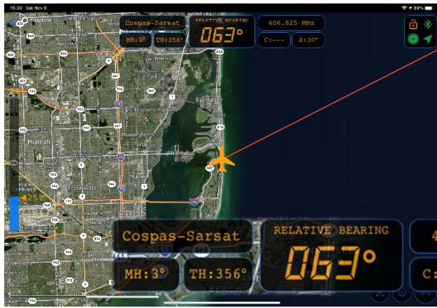
Prosecuting a Cospas-Sarsat beacon on 406.025 MHz with a REL LOB of 63°
