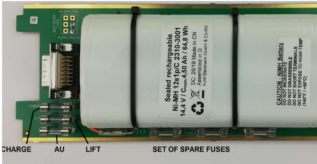
All input-and output connections are fused: Charge Input (CHARGE, 4 A slow-blow), Antenna Unit Output (AU, 1 A slow-blow) and Lift Output (LIFT, 0,5 A slow-blow). Additionally, spare fuses are provided.
