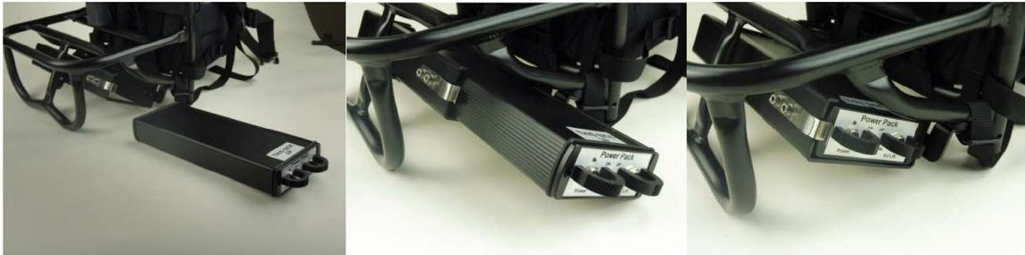
The power pack must be plugged into its rack as shown in the pictures above. As soon as the power pack is locked by the locking spring, it is automatically connected to the backward connector on the carrying frame and ready for use. To remove the power pack, pull the locking spring and unplug the power pack by pulling it forward.
