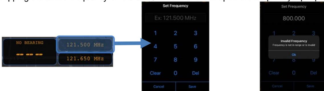
*Selecting an unavailable frequency causes an error appears*
