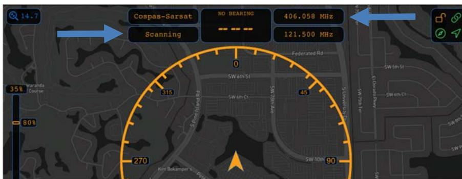
It is recommended to set 121.500MHz as the standby frequency because COSPAS-SARSAT usually transmits a strong long-range signal pulse approximately every 52 seconds. Typical COSPAS-SARSAT beacons emit a consistent low-range 121.500MHz signal, it's important to frequently monitor it for a continuous and accurate bearing.
