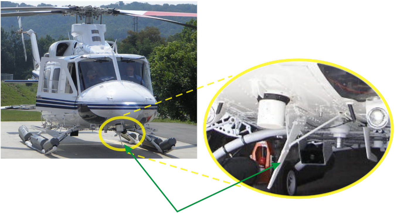
Fig 44) Antenna installed in a bad location
