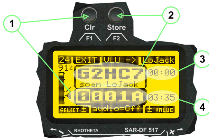
Fig 38) LoJack Scan Page with one active VLU Code and one new VLU Code
