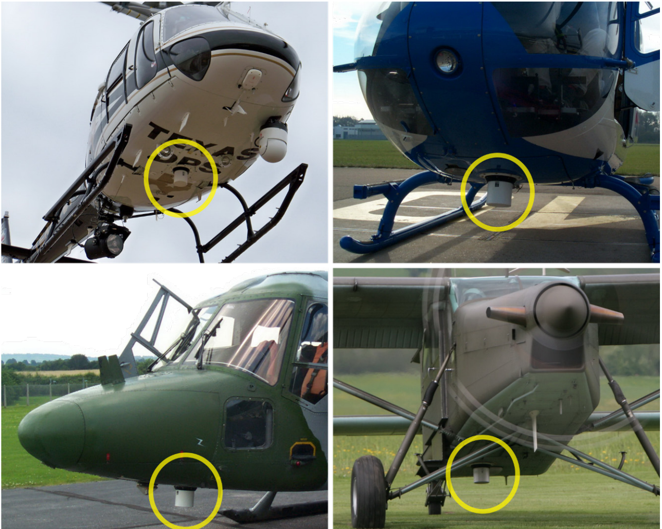
Fig 45) Antenna installed in good locations
