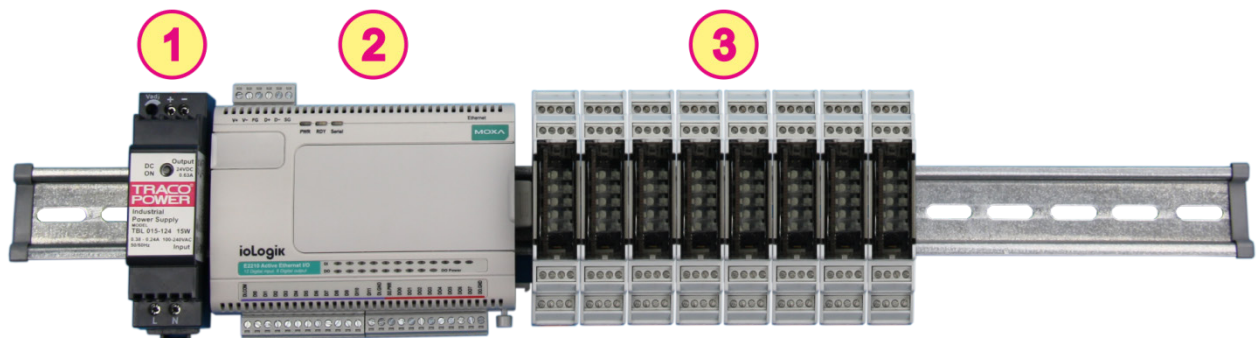
Figure 2: SNMP Module for RT-1000 Multichannel mounted on the 48.5 cm rack
