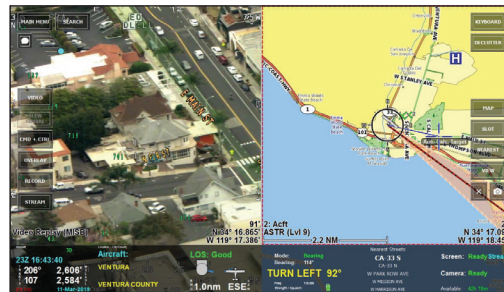
Digital mapping systems conveniently display DF information such as lines of bearing (LOB) labeled with transmitter ID, frequency, signal and squelch levels, estimated target location based on multiple LOBs, bearing cone indicating noise and reflections effects, lat long coordinates, etc. More DF control functionality will be increasingly added to the HMI of mission systems.
